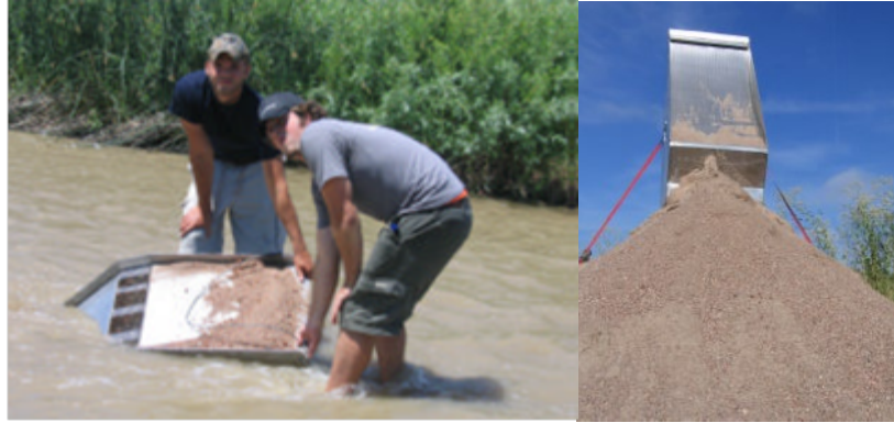
Figure 6. 2 ft (0.6 m) collector (left) and drop box (right) used to estimate production rates.
