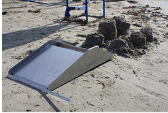
Figure 11. 2 ft (0.6 m) long Bedload Collector deployed on Galveston Island with harvested sand.
