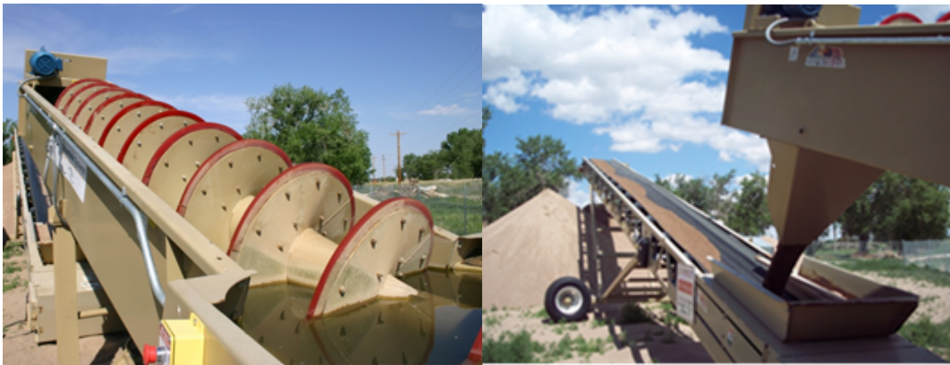
Figure 4. Sand washer (left) and radial stacker (right).
