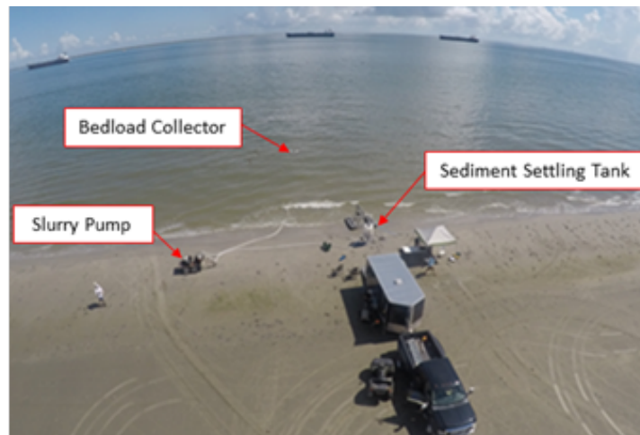
Figure 13. Scaled Bedload Collector pumping circuit (this trial being conducted at Big Reef Beach).
