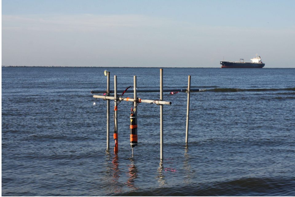
Figure 14. Doppler velocimeter (ADV) and optical backscatter sensor array collecting data at Big Reef Beach.
