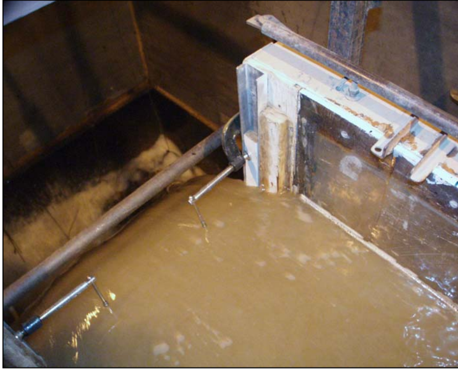
Figure 10. Photograph of Flow over Control Weir During Testing
