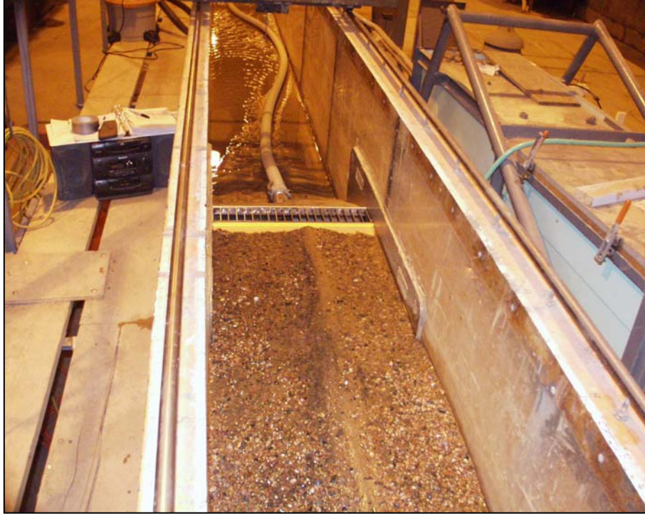
Figure 14. Photograph of Bed at Conclusion of Testing
