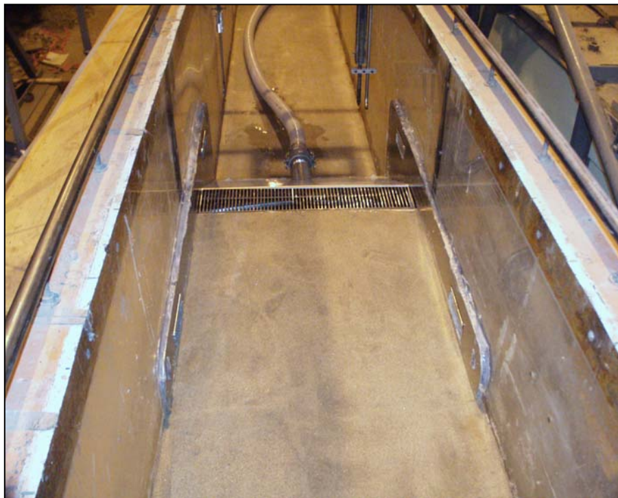
Figure 9. Photograph of BMC with Sand Bed in Place Prior to Testing
